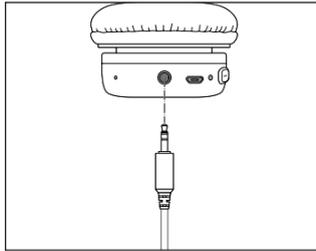
1. Connect the headphone output of the playback device to the audio connection port on the headphones using the AUX cable provided.
